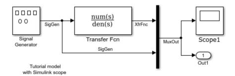
As you go through the tutorial, you transform ex\_slrt\_nrt\_osc into a Simulink Real-Time model configured to build as a real-time application. You then build, download, and execute the real-time application on the target computer.
