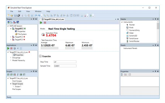
If you specify a sample time that is too small, a CPU overload can occur. If a CPU overload occurs, the target object property CPUOverload changes to detected. In that case, change **Fixed step size** to a larger value and rebuild the model.
